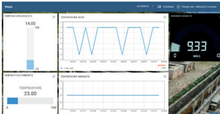
Figure 9. Dashboard or IoT platform applied to monitoring Source: own elaboration.
