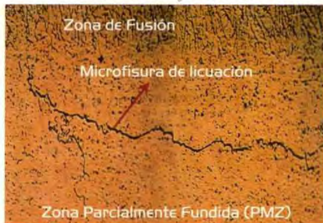
Figura 5 Micrografía Óptica (10 \mu m) AA6261T6/ER5356(2.08mg-0.51Si - 0.308Fe - , D=70.12% ; HI_3 = 3.33 KJ/ mm I_3 =165A 22V).
