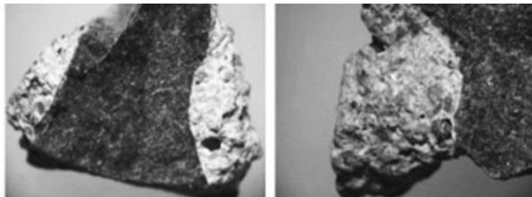
Figure 7. Coarse recycled aggregate particle morphology.
