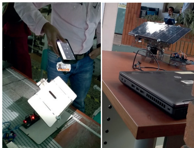
Image 5: tests with the prototype finalizing details and final version of the follower made in acrylic. Own source
