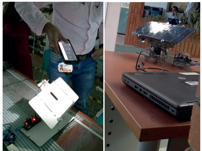
Image 5: tests with the prototype finalizing details and final version of the follower made in acrylic. Own source
